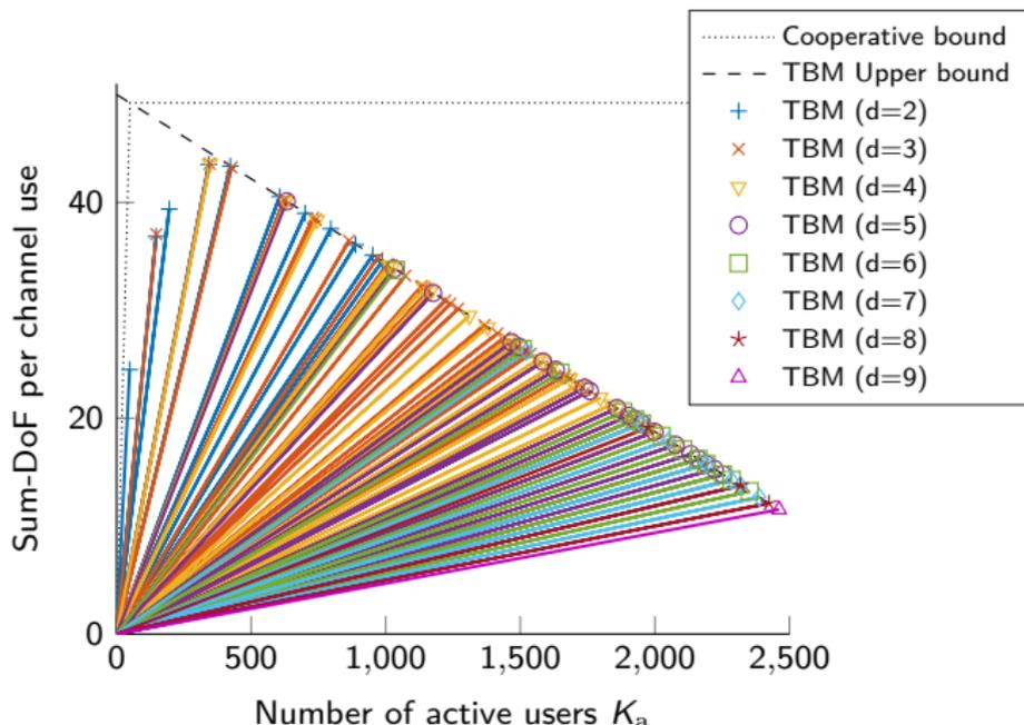
Achievable sum-DoF per channel use ( $D_{\text{TBM}}(K_a)/T$ ) vs.  $K_a$  for different tensor sizes ( $d$  and  $T_i$ ), for  $T = 3200$  and  $N = 50$  antennas.
